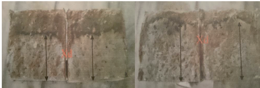
Figure 7: Penetration profounder of chloride ions; left) 25% substitution ; right) 0% substitution.
