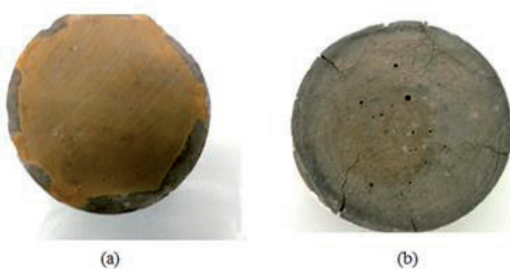
Figure 8: Comparison of observed damage of OCP samples after two months of sulfate exposure: (a) early age, (b) matured sample
